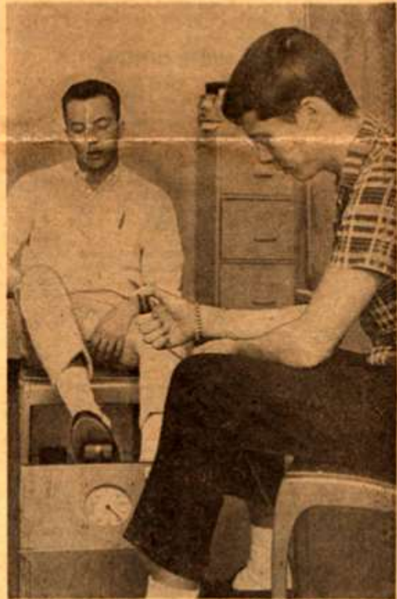
Gary Morris, right, gives Woody Zoll reaction test to see how fast Woody can get his foot off the accelerator and apply brake. Reaction time is registered on dial.
